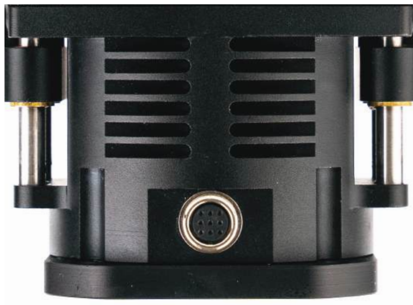
Figure 2.4 - Communication port on the SusGrip gripper
