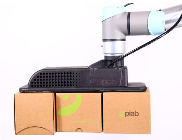
By enabling multipicking of boxes, the CPT enables palletizing processes to reach a new level of efficiency.
