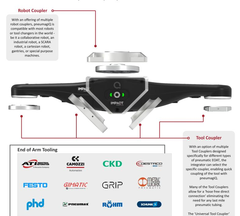
pneumagiQ has been built as a 'platform' enabling to simplify the implementation of pneumatic end of arm tooling.
