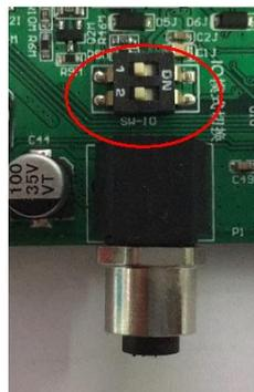
The DIP switch 1 controls the Output pin hardware of the protocol converter in the I/O mode.
