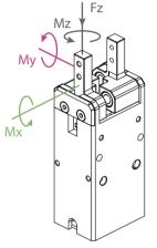
Allowable vertical load (static)
