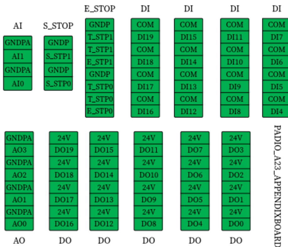
Figure 7-2 : The layout of the electrical interfaces inside the controller
