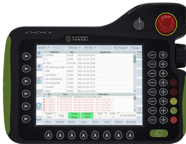
Figure 1-1 : Emergency stop button
