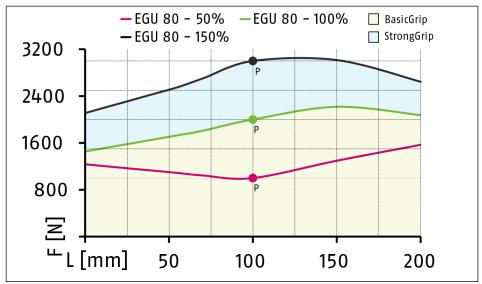
Gripping force diagram EGU 80 M (with Gripping force and position maintenance (GPE))
