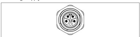
EGU - PWR PIN allocation connector, voltage supply
