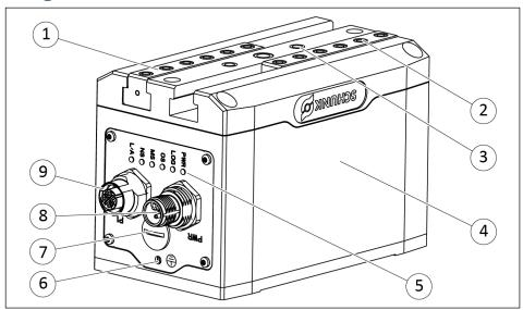
Universal gripper, electric EGU, example variant PROFINET
