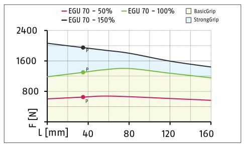
Gripping force diagram EGU 70 M (with Gripping force and position maintenance (GPE))
