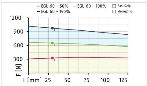
Gripping force diagram EGU 60 M (with Gripping force and position maintenance (GPE))
