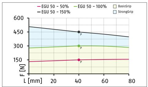
Gripping force diagram EGU 50 M (with Gripping force and position maintenance (GPE))
