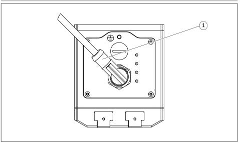
Cable outlet, example 10-Link, Modbus RTU
