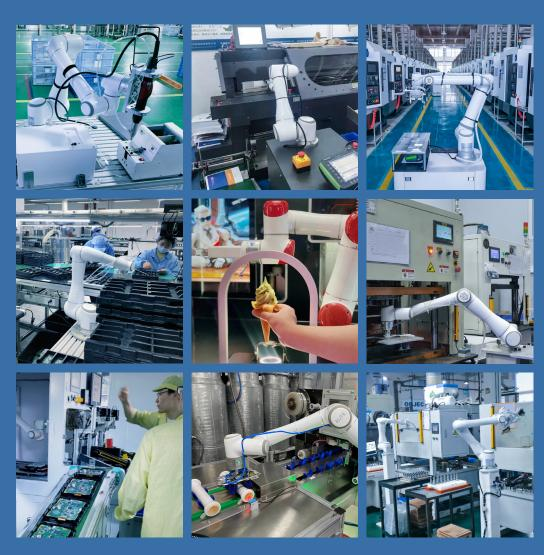
Intended applications include material handling, locking screws, testing, coating, material removal, handling, palletizing and other production tasks.
