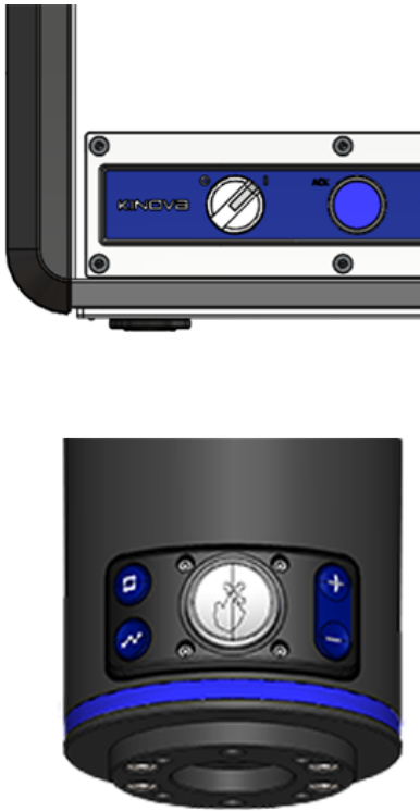
Figure 78: Visual cues of robot in Monitored stop
