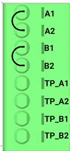
Figure 36: Terminal connections with jumper wire on A1, A2, B1, and B2 when the teach pendant is connected
