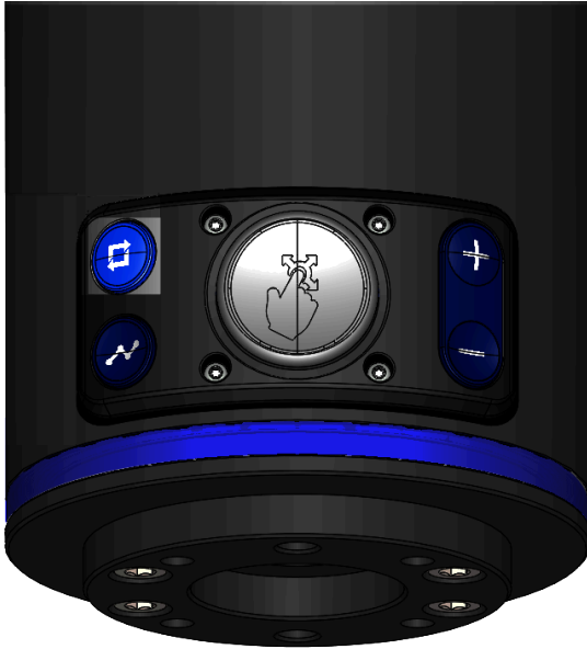
Figure 87: Location of Hand Guiding mode Toggle on the wrist
