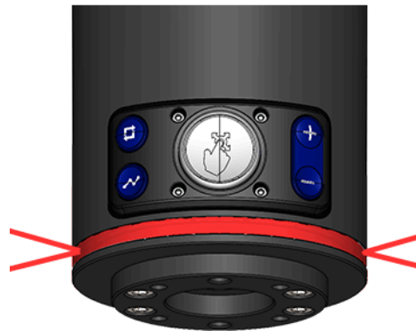
Figure 80: Visual cue of fault with power
