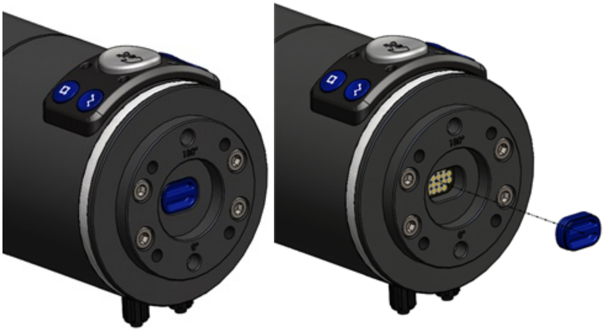
Figure 14: Central connector on wrist with cap on and with cap off
