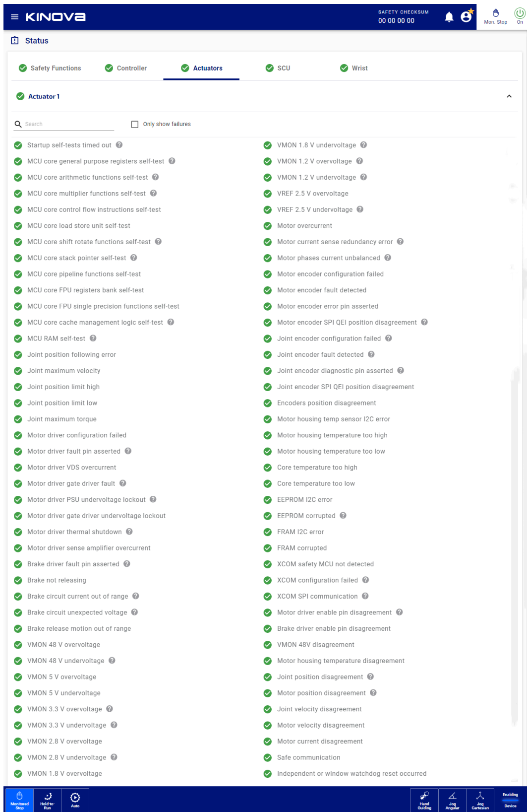
Figure 218: Status page of the actuators with an actuator pane expanded
