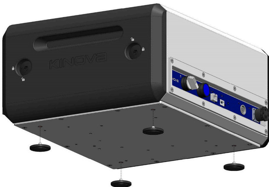
Figure 22: Mounting points of the controller
