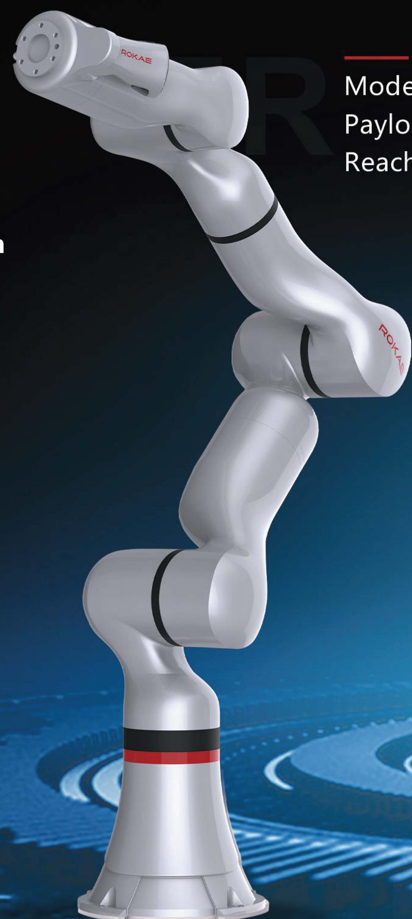
Model ER7 Payload 7kg Reach 1,125mm
