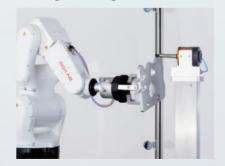
Grinding and deburring of cast iron parts, aluminum and magnesium alloy die-cast parts, and steel machined parts
