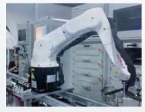
Loading and unloading for inspection equipment of mobile phones and other electronic products
