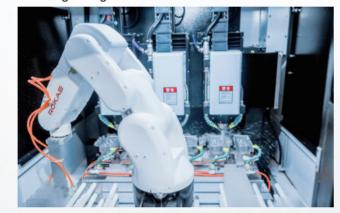
Loading and Unloading for Injection Moulding Machine
