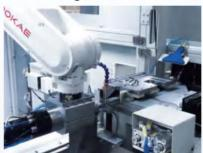
Chamfering and deburring of different end surfaces of auto linear guides
