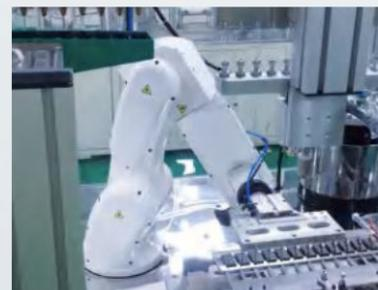
Encapsulating and gluing of relays and other electronic components
