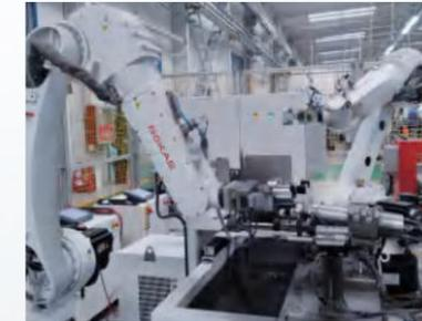
Fine grinding and deburring of piston products (including valves, oil holes, inner pin holes, and other complex parts)
