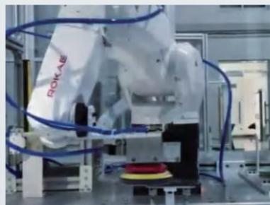
Grinding and polishing of the metal backboards of mobile phones and other electronic products
