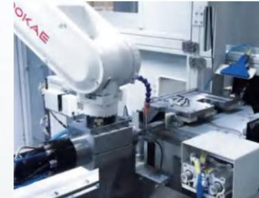
Chamfering and deburring of different end surfaces of auto linear guides
