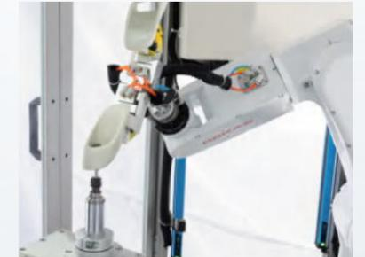
Grinding and polishing of interior and exterior plastic trims, such as door handles and three-spoke steering wheels
