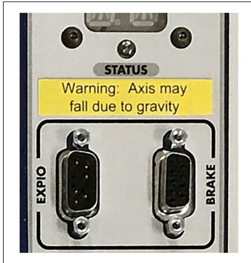
Figure 12-2. Brake-release/Gravity Warning Label
