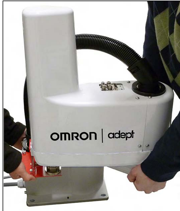
Figure 3-3. Lifting the Robot
