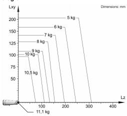
The KR 10 R1100-2 is designed for a rated payload of 5 kg in order to optimize the dynamic performance of the robot. With reduced load center distances and favorable supplementary loads, a maximum payload of up to 11.1 kg can be mounted. The specific KUKA Load case must be verified using KUKA. For further consultation, please contact KUKA Service.
