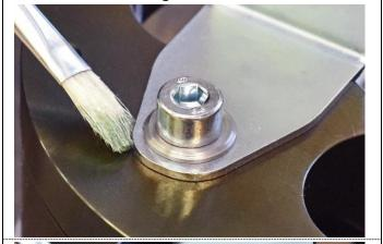
Apply a small amount of grease (Molykote BR2Plus) on the surfaces between the hose/cable guide and the CiRo-shaft and the hose/cable guide and the bushing, respectively.
