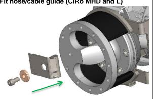
Fit the hose/cable guide, bushing and enclosed screw to the CiRo.
