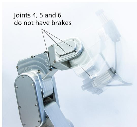
Figure 4: When the robot is deactivated, the end-effector will slowly move downwards under the effects of gravity
