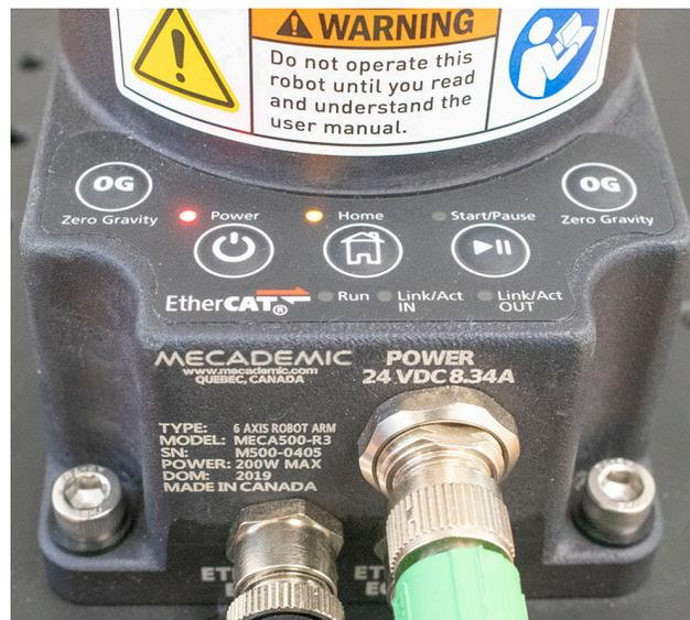
Figure 20: Robot control panel
