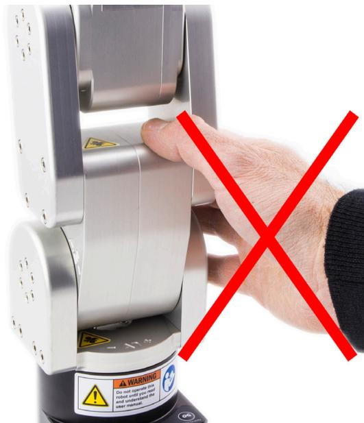
Figure 1: Pinch point example
