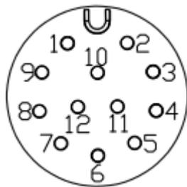
Fig. 36 Definition of PS1 pins
