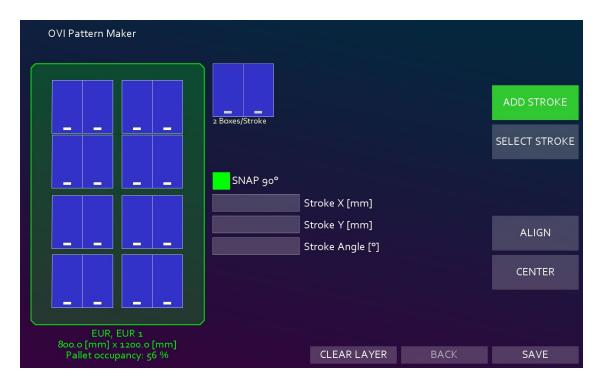
**Step 7**: The pattern can be edited by pressing the "SELECT STROKE" button and then clicking on an existing stroke (box or group of boxes) from the pattern on the left side.
