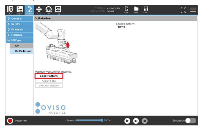
An XML file containing a palletising pattern can be loaded by pressing the "Load Pattern" button on the left hand side of the user interface (UI).
