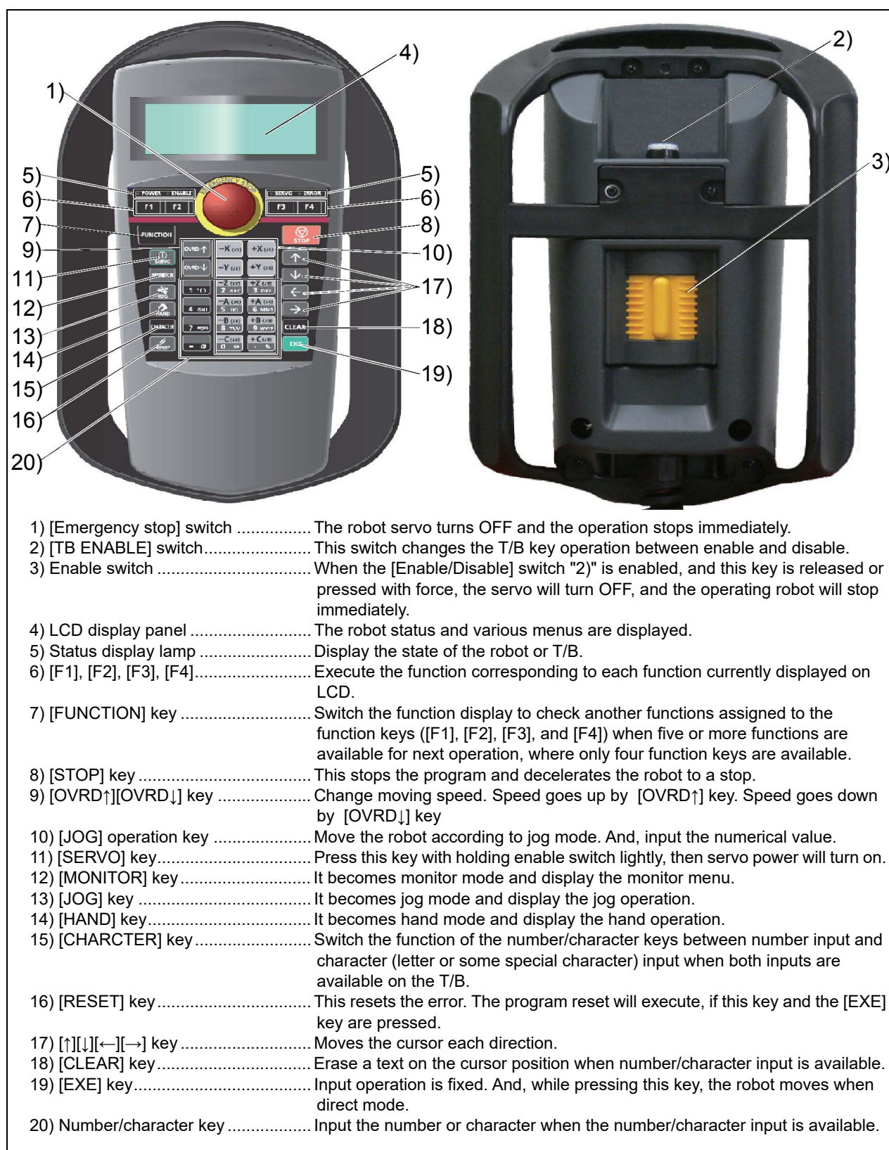
Fig.3-17: Teaching pendant key layout and main functions
