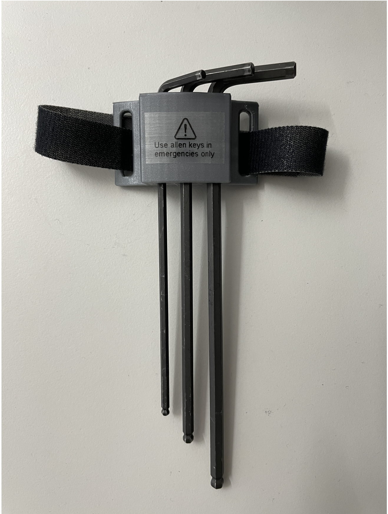
The allen keys to open the clamps and disassemble the modular configuration
