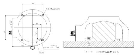
Figure 12. Reference bracket fixing method
