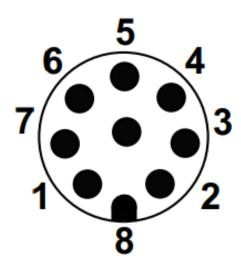
Figure 28. The wrist round connector interface
