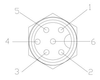
Figure 26. The EtherCAT debug interface
