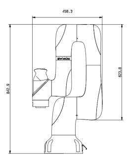
Figure 11. Reference transportation dimensions of the robot
