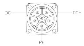
Figure 16. Power supply interface
