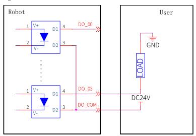
Figure 22. NPN output wiring diagram
