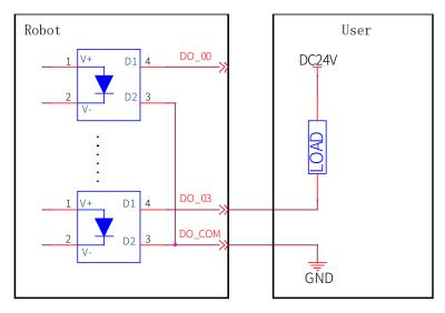
Figure 21. PNP output wiring diagram
