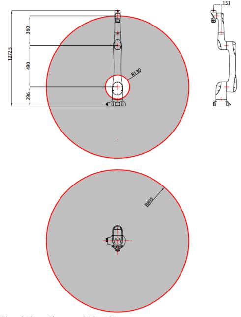
Figure 8. The working space of xMate CR7
