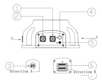
Figure 15. Base interface layout
