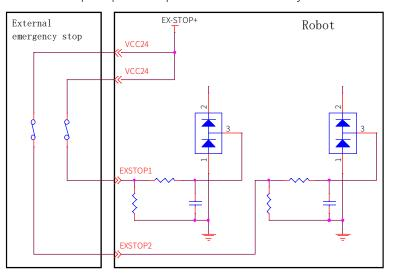
Figure 23. External emergency stop interface
