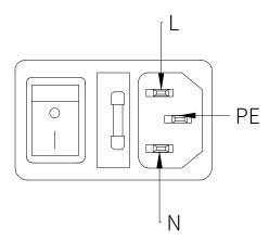
Figure 32. Power input interface
