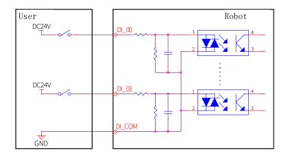
Figure 19. PNP input wiring diagram
